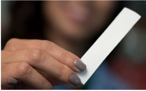
The explosive-detecting paper strips are coated with tiny semiconductor particles known as silicon quantum dots. Image 1 of 2
